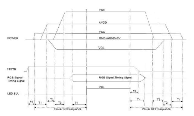
Note: T1≥20ms, T2≥20ms, T3≥5ms, T4≥100ms, T5≥5ms, T6≥5ms.
