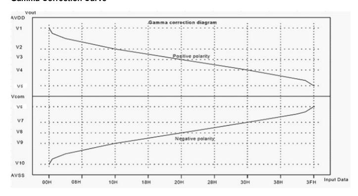
**Gamma Correction Reference Voltage Setting**
